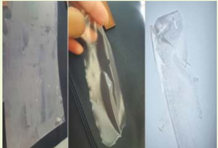
Biopolymer is spread over a thin sheet to form its Dried bioplastic
