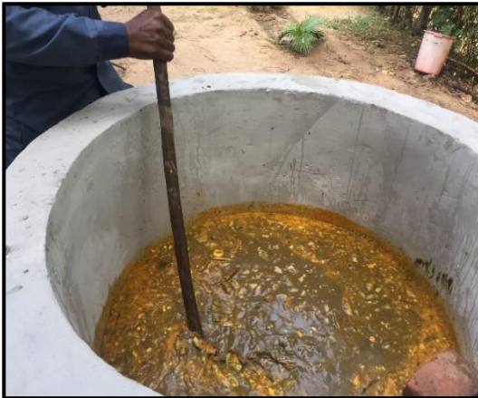
Addition of Cow dung to Initiate the Production of Biogas
