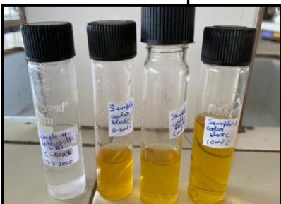
Sample-4 and 5 : Yellow Color with no gas ; Potable water
