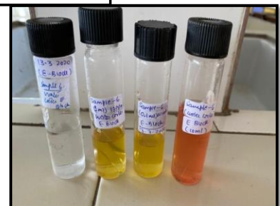
Sample-6 : No gas with slight color change ; Potable water
